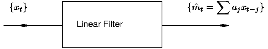
Figure 1-20 Smoothing with a low-pass linear filter.
